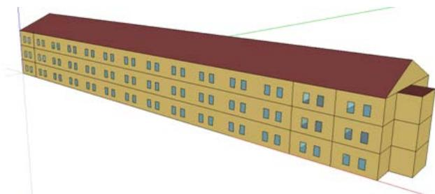
**Figure 4 Barracks model (WWR=9%, SRR=0%)**
