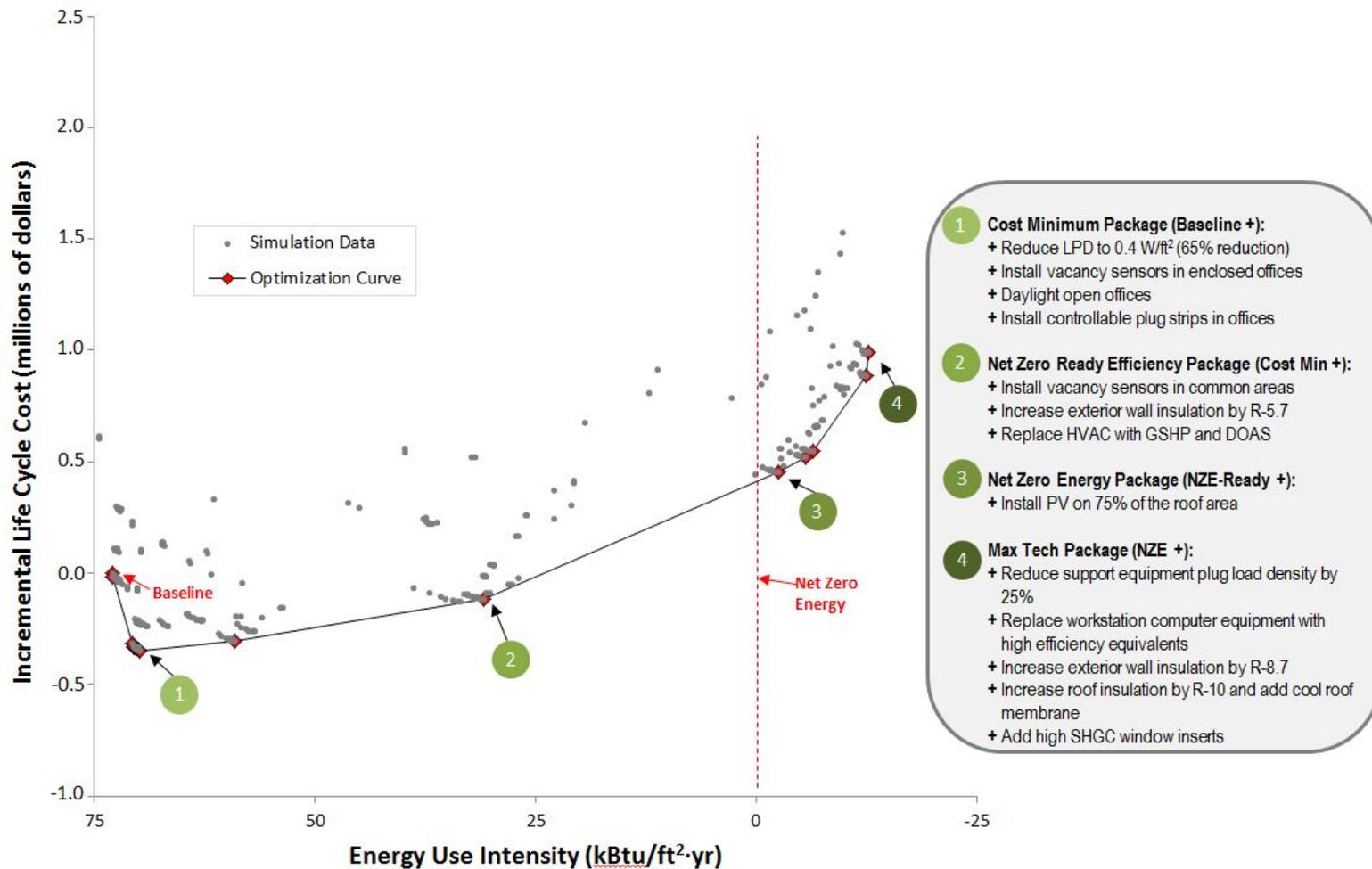
Note: DOAS – dedicated outdoor air system, GSHP – Ground source heat pump, HVAC – heating, ventilation, and air conditioning, kBtu/ft<sup>2</sup>·yr – thousand British thermal units per square foot per year, LPD – Lighting Power Density, PV – Photovoltaic, SHGC – Solar heat gain coefficient, W/ft<sup>2</sup> – watts per square foot
