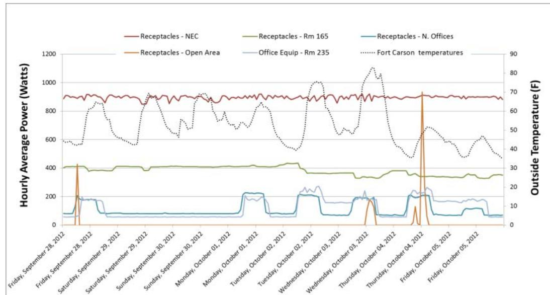
**Figure 79 Hourly average power draws for several plug loads in Building 1219**
