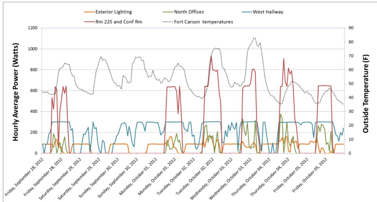
**Figure 80 Hourly average power draws for a sample of lighting circuits in Building 1219**
