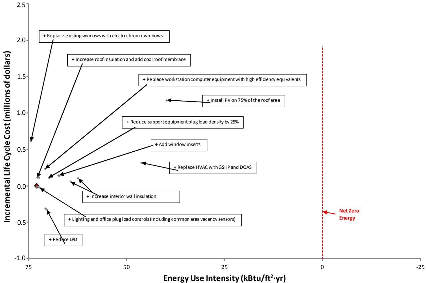
Figure 46 Baseline model and first iteration of perturbations
