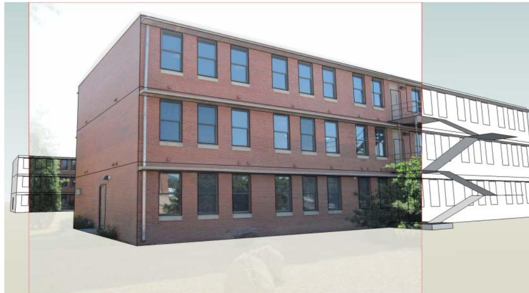
**Figure 42 Specify exterior geometry using Match Photo**
