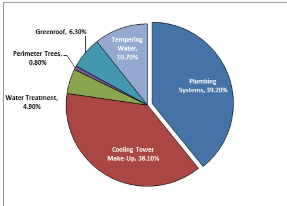
Figure 5-5. Potable Water Use at Wynkoop Building—2011
