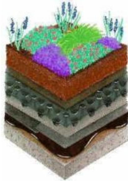
Some changes were made to the roof assembly to accommodate this system. The building's roof is an EPDM membrane with a high-emissivity acrylic coating; the membrane was changed from 60 mil to 90 mil, a fleece protection mat was added to protect the membrane from friction, and the warranty was extended from 10 to 15 years. Recycled rubber pavers provide walking paths around the perimeter of the modular systems for use by maintenance personnel.
